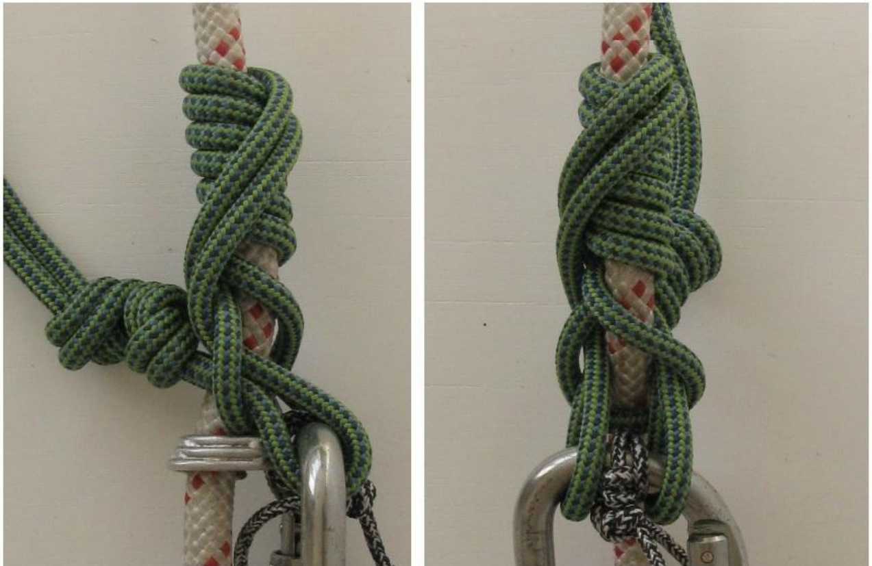
Figure 2.8; Photo of HAH friction hitch, loop version, with tending ring
