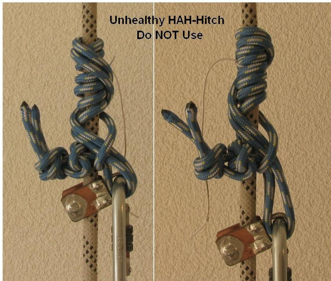
Figure 2.6; Photo of unhealthy HAH friction hitch (too much slack)
