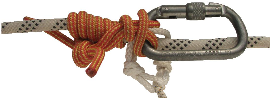
Figure 2.3; Hedden Friction Hitch as progress capture device
