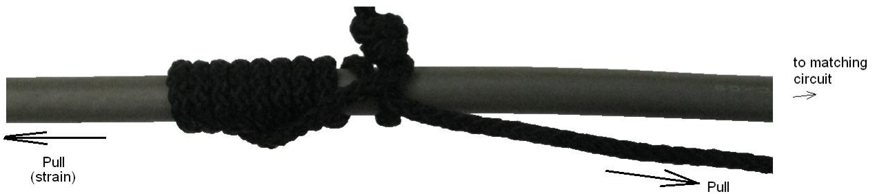
Figure 8.9.5, friction hitch for strain relief, alternative
