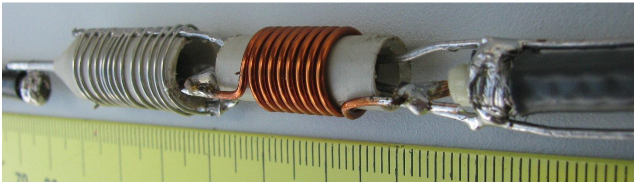
Figure 8.7.4: Detail of matching circuit.
