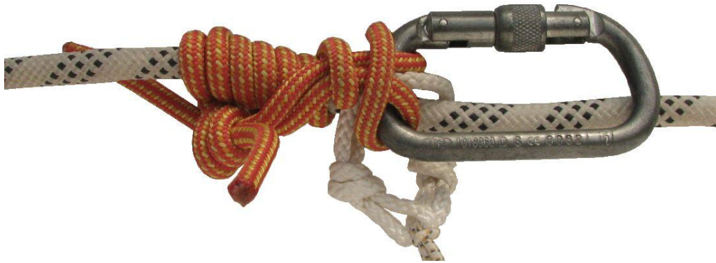
Figure 5.6.2: 4 turns Hedden Friction Hitch with low backlash
