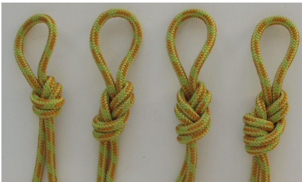
Figure 4.9.1, Overhand, figure 8, 9 and 10, all on a bight
