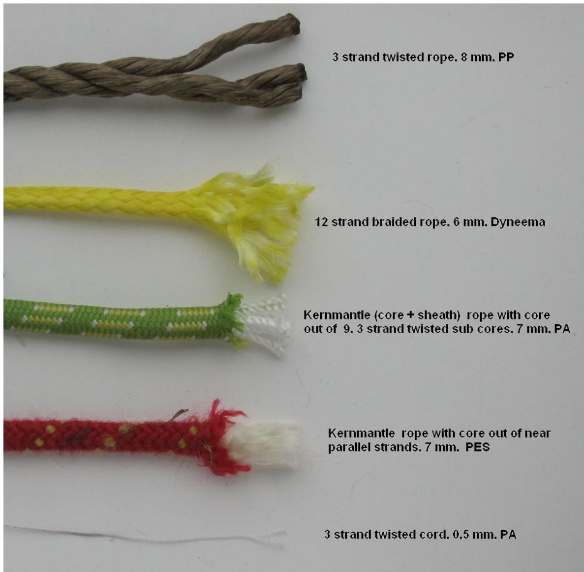
Figure 2.1, various rope/cord constructions
