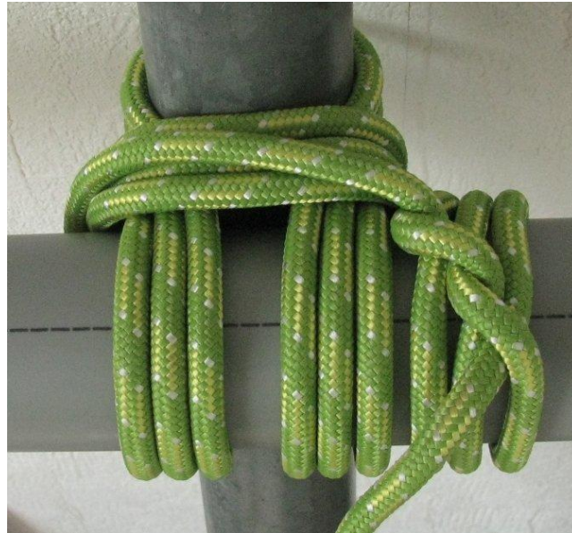
Figure 8.17, photo of complete square lashing
