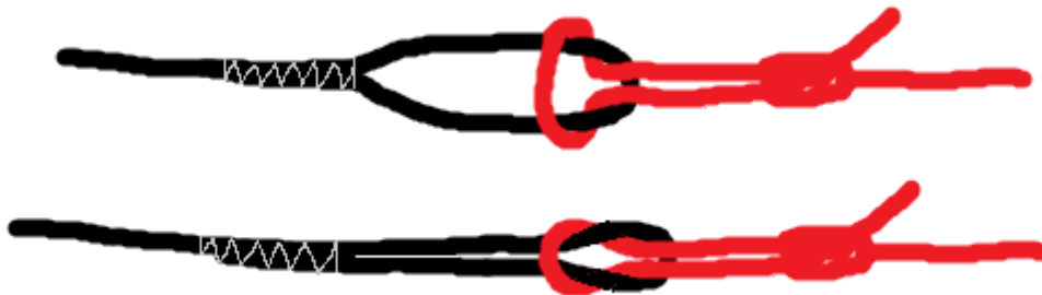
Figure 4.15, Bend using two eye terminations
